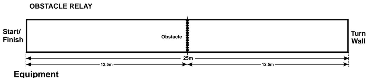
**Obstacles:** The obstacles used for competition should be appropriate for pool depth and will easily allow athletes to pass under. 70 cm high obstacles should be used with a minimum pool depth of 1.8 m, while the smaller 35 cm high obstacles should be used with a minimum pool depth of 1.2m. Obstacles are fixed at a right angle onto lane ropes in a straight line across all lanes. The obstacle is located 12.5 m from the starting edge.
